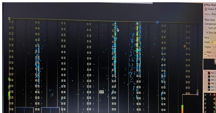
Figure 8. congestion map after creating partial blockages of size 10 \times 10 \mu\text{m}^2
