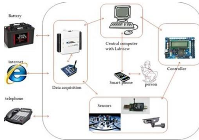
Figure 2. Block diagram of the entire system
