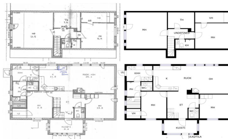
Fig. 2. Sample images from Cubicasa 5k dataset. The images from left to right are original floorplan image and the SVG label. [4]
