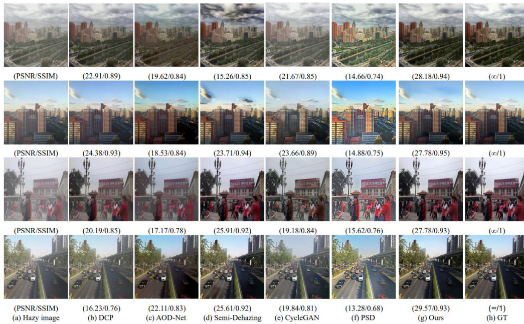
Figure 2. Image dehazing results on the SOTS outdoor dataset. From (a) to (h): (a) the hazy image, and the dehazing results of (b) DCP [8], (c) AOD-Net [33], (d) Semi-Dehazing [41], (e) CycleGAN [37], (f) PSD [40], (g) Our WTCL-Dehaze and (h) ground-truth image respectively. Our method generates cleaner results with fewer artifacts and minimal color distortion.
